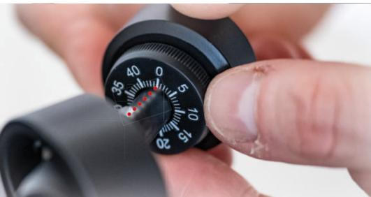
**17** Turn the whole counterweight counter-clockwise until the scale reads 18 - 20.
